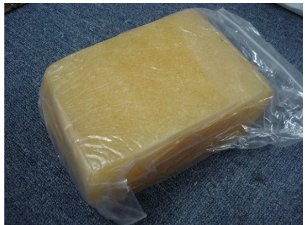
Figure 2: SBR 1502 is a general-purpose grade of synthetic rubber, often used in blends with other rubber types.
